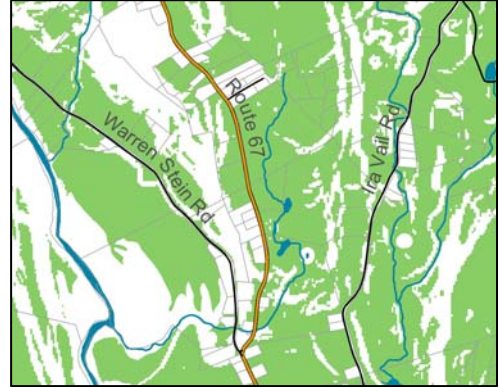
Figure 6: After removing the environmental constraints from the buildable parcels, these buildable areas are left (in green).
